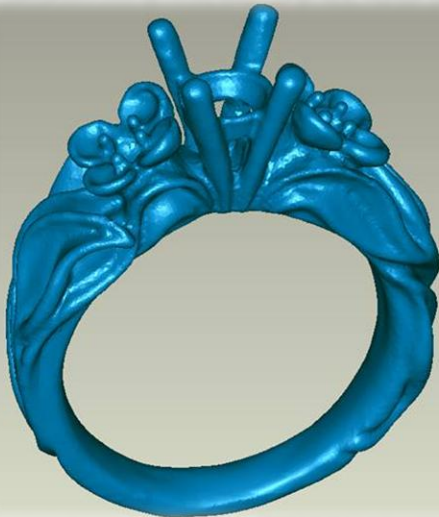
Watertight .stl mesh used to print high resolution wax model used for investment casting.
